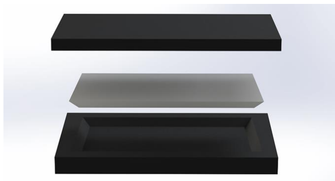
The seat cushion is made up of three different types of foam.
