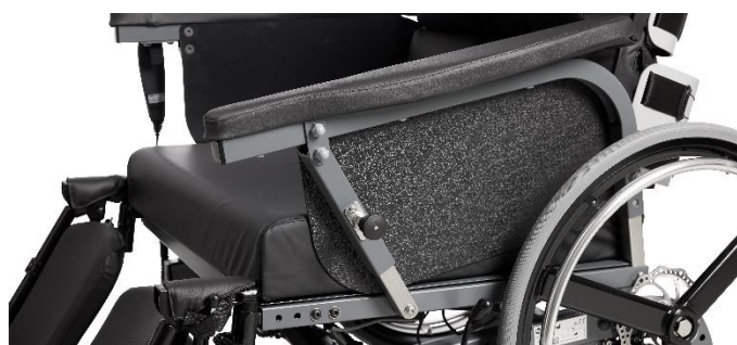
Swivelling armrests allow positioning near a table.
