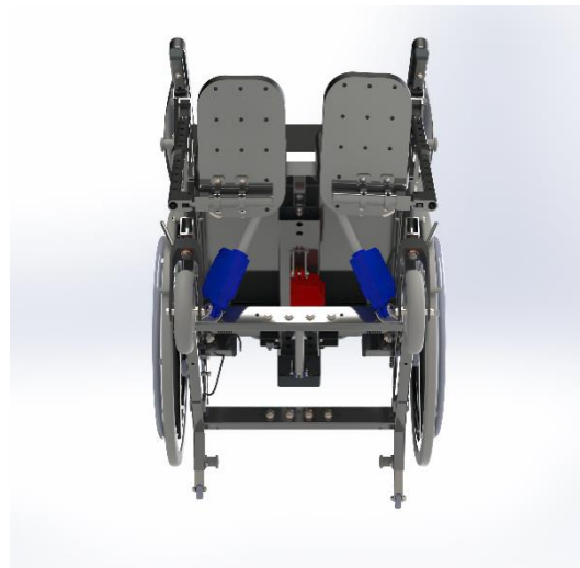
Two actuators (marked blue) control the tilt-in-space function. One actuator (red) controls the recline function.
